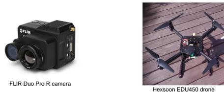
The images were collected using FLIR Duo Pro R camera which has an IR lens and an RGB lens. The IR lens has a resolution of 640 x 512 (0.3 MP), 1.33 aspect ratio, 13 mm focal length, and temperature range -40°C to +550°C. The RGB lens has a resolution of 4000 x 3000 (12 MP), and an 8 mm focal length. The images will be collected using a Hexsoon EDU450 drone which was built by the members of NEIL.
