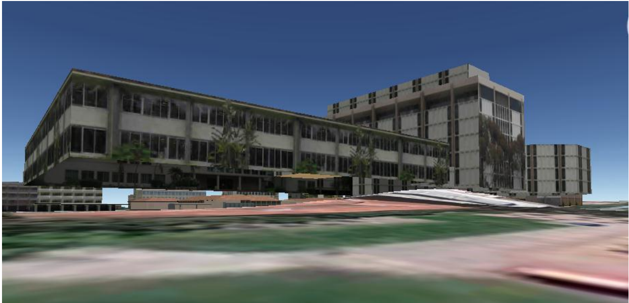
Figure 1: An error in the underlying DEM causes the Davidson Library on the UCSB campus to appear to float 6 meters above the ground within Google Earth. This type of error highlights the need for enhanced ground filtering algorithms such as SMRF.
